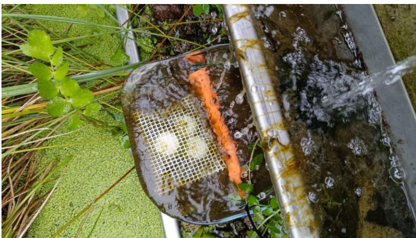
Figure 24. Picture showing the deployment of DGTs (white) and VPS (orange) in the NBS.
